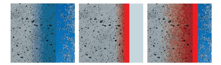
Untreated concrete is a porous system, which is prone to water penetration.
