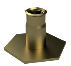
The HALFEN TWS Hexagon plate anchors are used as auxiliary aids when erecting precast elements. For example, temporary anchor points for push-pull props for fixing twin-walls to in-situ concrete floor slabs and foundation slabs. The hexagon plate anchor is suitable for wind loads and other temporary loads.
