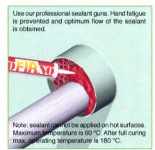
5) A 20 mm thick layer of NOFIRNO® sealant is applied at each side of the con-duit. Clean and dry the conduit opening as well as the pipe thoroughly, and remove any dirt, rust or oil residues before applying the sealant.
