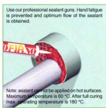
5) A 20 mm thick layer of NOFIRNO® sealant is applied at each side of the con-duit. Clean and dry the conduit opening as well as the pipe thoroughly, and remove any dirt, rust or oil residues before applying the sealant.
