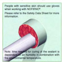
6) The conduit should be overfilled with NOFIRNO® sealant, because some sealant will be pushed between and into the empty filler sleeves during further finishing. This will contribute to obtain higher tightness ratings.
