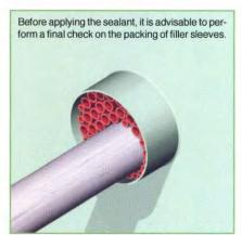
4) Push the filler sleeves into the conduit in such a way as to leave about 20 mm free space at the front. The whole set of filler sleeves should tightly fit into the conduit to provide sufficient mechanical stability.
