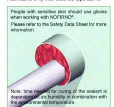
6) The conduit should be overfilled with NOFIRNO® sealant, because some sealant will be pushed between and into the empty filler sleeves during further finishing. This will contribute to obtain higher tightness ratings.
